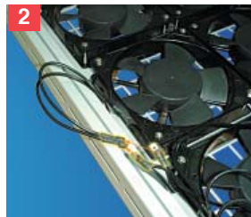
2 adjust wire pin to aim at connector Housing
